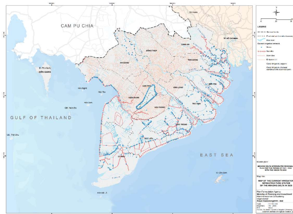
Figure 2-2 Water management infrastructure – rivers and canals, river and sea dikes, and existing sluice gates in the Mekong Delta in Viet Nam (MDIRP, 2022)
